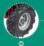
DRIVE WHEELS tractor profile with mechanical semidifferential
